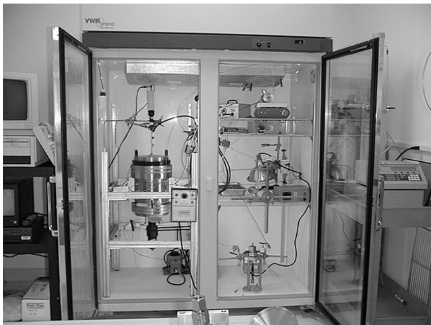
Figure 9 Liquid CO 2 spin coating apparatus.
